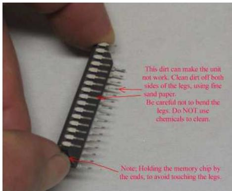
Before putting the old program memory chip in the new keypad, you should clean the dirt off the legs of the memory chip. You can use very fine sand paper to do this. **Do NOT use any chemicals on it.**
