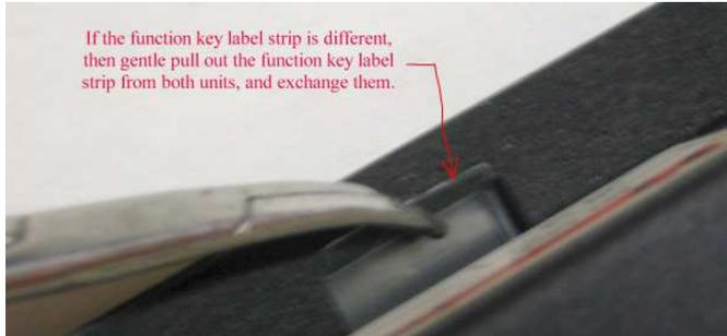
Start with the new keypad; Turn the keypad over to see the backside again. You should see a small piece of clear plastic sticking up through the foam insulation on the right side of the keypad. Using your fingers (or tweezers if you can't reach it) gently pull the function key label strip out.
